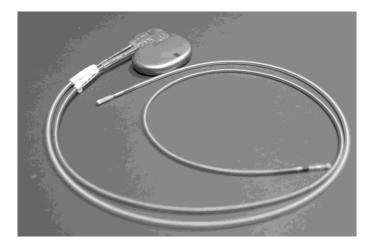
The pacemaker system is comprised of a pulse generator (or battery box) and one or more electrode leads depending on the nature of your heart condition:
